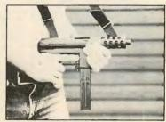
Photo sequence shows newly imported semiauto machine pistol, the Interdynamic KG-9. Manufactured in Sweden, the KG-9 incorporates features of the Schmeisser, M-3 Greasegun, and Swedish Carl-Gustav. Chambered in 9mm Parabellum, this new weapon weighs in at 67 ounces when fully loaded with 32 rounds. Length is just over one foot, including the five-inch barrel.
